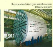
Reverse circulation type shield machine (Stage 2 project)
