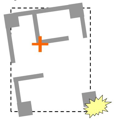
Eccentricity ratio: Balance of each floor's stiffness in horizontal plane
