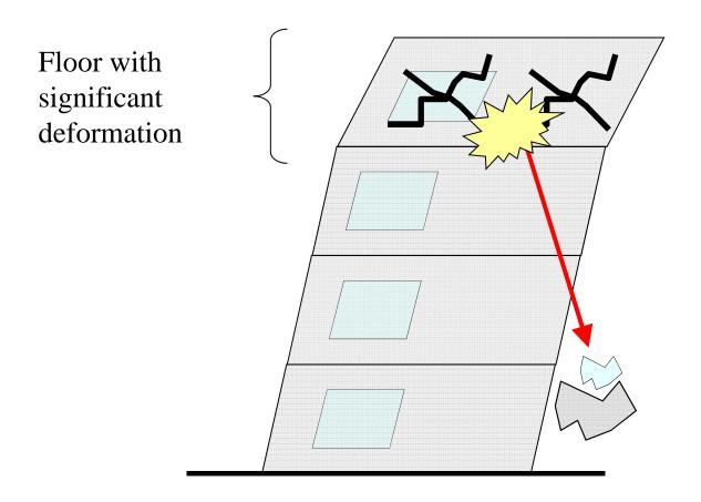
Story deformation angle: Deformation of each floor
