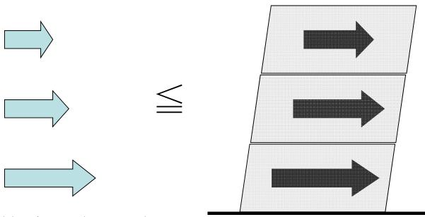
Required horizontal strength: Horizontal strength required for each floor in the event of a large earthquake
